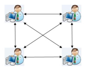
In an environment where it was deemed desirable to cater for many different vendor products, multiple inter-communication protocols would be needed (possibly one unique protocol per vendor product). This would result in the configuration shown on the left.
